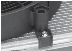
Radiator Frame Rail Mounting
