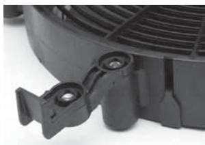
Radiator Frame Rail Mount with Extender
